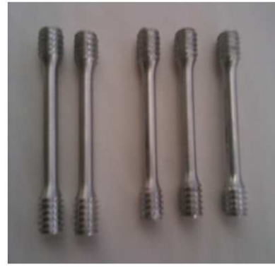
Figure 9: Photograph of SCC Test Specimen
