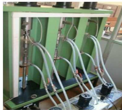
Figure 11: View of Salt Water Circulation
